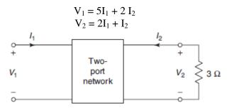
A load resistor of 3  $\Omega$  is connected across port 2. Calculate the input impedance.
